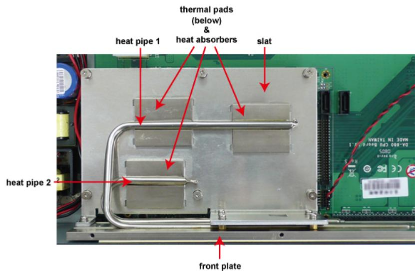
For example, silicon thermal pads can be used to directly cover the onboard CPU and chipsets, which are then covered by aluminum heat absorbers located on the slat where one or more bronze heat pipes are affixed. The heat pipes are hollow but lined with a wick containing a working fluid, such as water,
