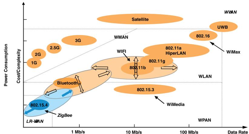
As you can see, these technology options roughly show the relationship between the data communication rate (data rate) and complexity of implementation: the higher the data rate required in the wireless application, the more cost and power consumption it may take. Therefore, you will need to select the most appropriate solution for your wireless network.
