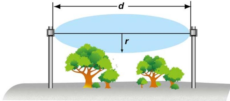
$$r_{(\text{in mts})} = 17.32X \sqrt{\frac{d_{(\text{in km})}}{4f_{(\text{in GHz})}}} \quad r_{(\text{in ft})} = 72.05X \sqrt{\frac{d_{(\text{in km})}}{4f_{(\text{in GHz})}}}$$
