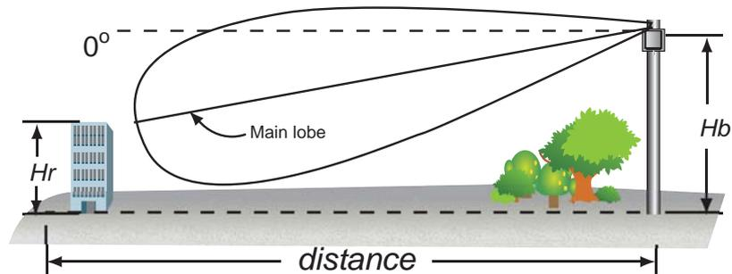
$$\text{distance} = \frac{(Hb - Hr) / \tan A}{5280} \quad \text{angle} = \tan^{-1} \left( \frac{(Hb - Hr)}{\text{distance} \times 5280} \right)$$
