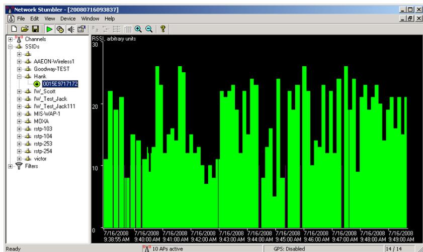
You can download this utility from Network Stumbler ([www.netstumbler.com](http://www.netstumbler.com)). The following general steps should be followed when performing a site survey. Remember, the objective of the survey is to identify potential sources of interference in the target environment and determine the best locations for your access points.
