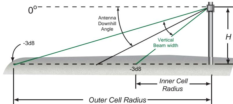
$$\text{Inner Radius Distance} = \frac{H/\tan(A + \frac{BW}{2})}{5280} \quad \text{Outer Radius Distance} = \frac{H/\tan(A - \frac{BW}{2})}{5280}$$
