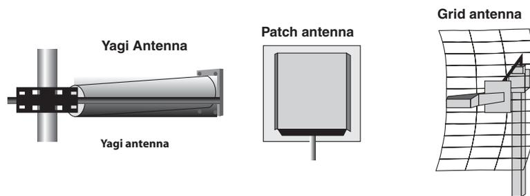
If you are planning to extend the range or widen the coverage, you may need to use external high-gain antennas for your access points. In addition to the antenna type and gain, you need to pay attention to the following specifications:
