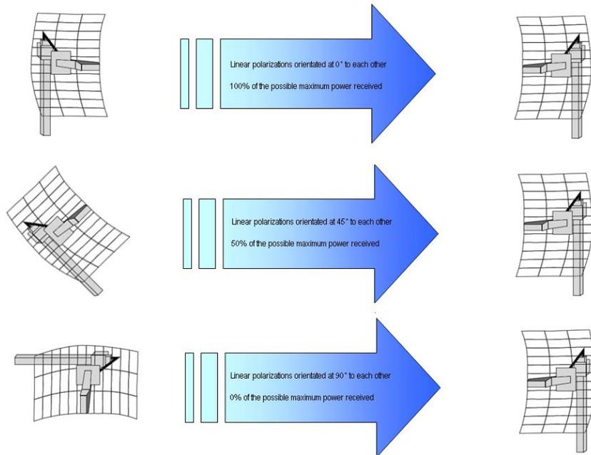
Utilizing antenna polarization can also help make your wireless network more robust. For example, you can install your antennas vertically in an area with mostly horizontal antenna installations, as shown in the following figure, in order to reduce interference.
