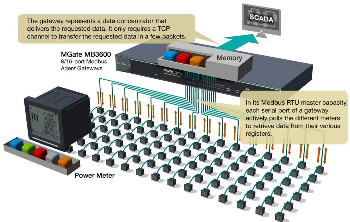
For any system integrator, easy configuration is always a high priority. In agent mode, the gateway in its RTU master capacity can set many Modbus commands. In order to save time with configuration, some gateway brands support comma-separated value (CSV) files, which can be easily configured and imported into the gateway by using excel.
