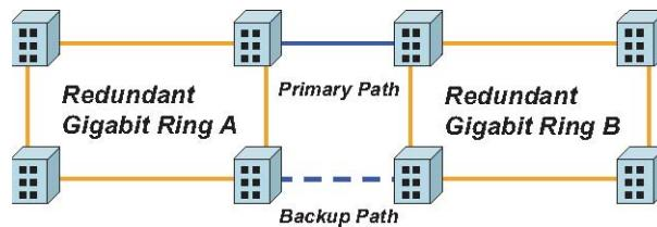
In this figure, ring coupling is illustrated with two lines connecting Ring A and Ring B. One line is the primary path, and the other is a redundant backup path. Field Switch C needs an additional gigabit port to build these two paths, for a total of three gigabit ports for ring coupling, or four gigabit ports if an additional uplink port with the core switch is needed.
