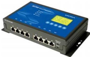
Moxa's UC-7400 is a RISC-based Universal Communicator that uses a Linux OS, and comes with 8 Serial Ports, Dual Ethernet ports, USB, PCMCIA, and CompactFlash. The following features make UC-7400 an excellent choice for your industrial front-end computing applications:
