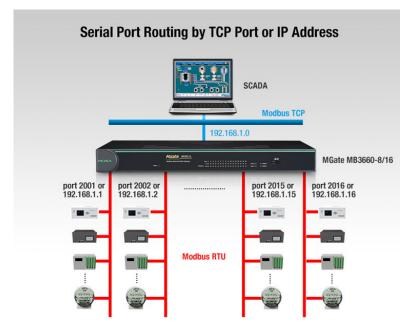
Furthermore, serial-port mapping with IP addresses or TCP ports needs to be manually maintained by an engineer, which requires the engineer to identify the serial port that a device is connected to, and the corresponding IP address or TCP port.
