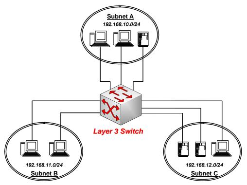
In the figure, we show a layer 3 switch connected to switches and hosts from the three subnets. Since the layer 3 switch uses IP addresses to direct traffic, it is capable of transmitting packets from any network host on the LAN to any other network host on the LAN.
