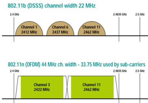
In the following sections, our discussion only includes the 2.4 GHz band and 5 GHz band because they are the most commonly used bands in WLAN applications. In addition to IEEE 802.11 standards, the tradeoffs between these two bands are usually considered with interference (almost entirely in the 2.4 GHz band) and range (bigger power loss shortens the transmission distance in the 5 GHz band).
