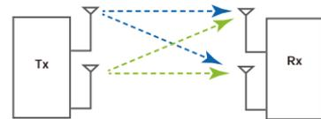
When multiple transmitters and multiple receivers are used, simultaneous data streams can be sent, which increase the data rate. In addition, multiple receivers allow greater coverage and longer distances between devices. The IEEE 802.11n standard uses MIMO to increase speed to 100 Mbps and beyond. MIMO technology is also used in LTE and other wireless standards.
